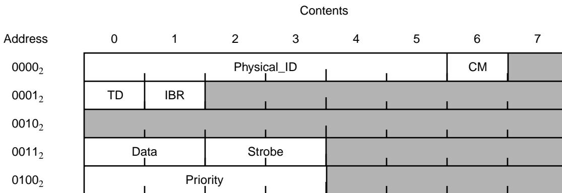
Figure 5B-4 — PHY register map for the backplane environment
